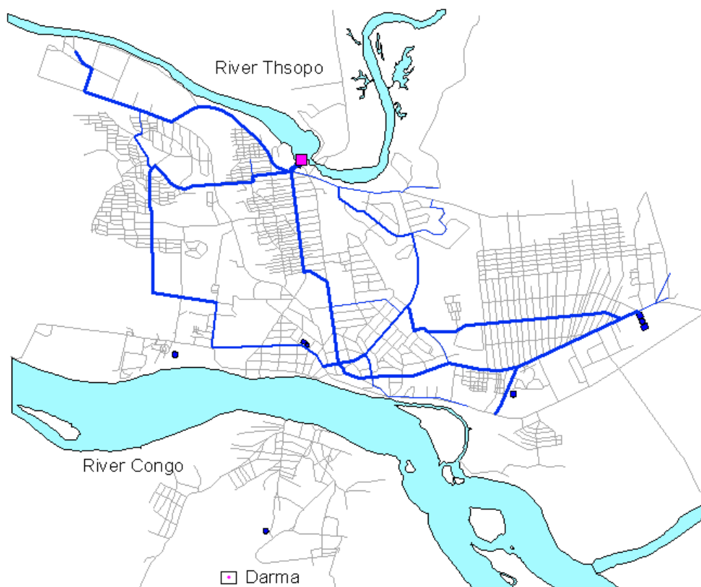
Figure 1 Kisangani Map of the town, of the road grid and location of the 2 water treatment stations, the primary network grid and the main storage reservoirs.
